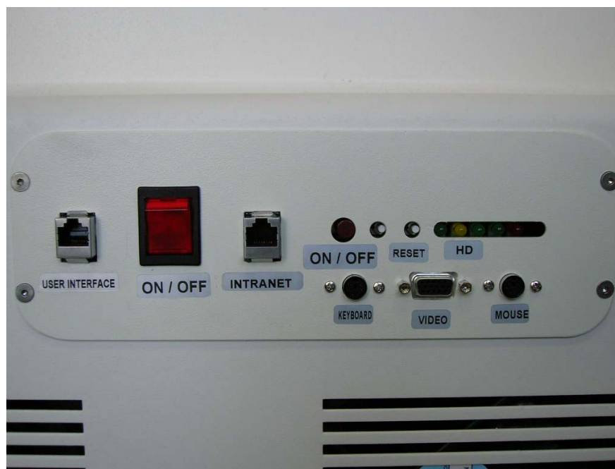
Figure 3. Rear of VISTA-CT scanner. Main ON/OFF switch is the large RED switch on the left.
