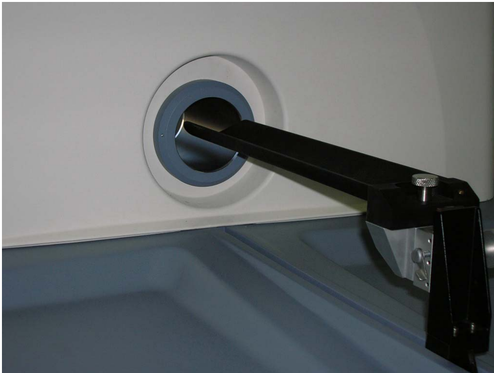
Figure 1. Animal bed, vertical bed movement mechanism and gantry aperture.
