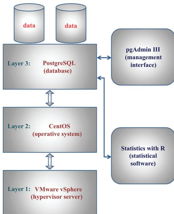
**Fig. (1).** Software architecture of the system completely open source.
